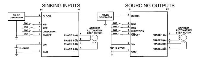
With JP1 in position 1-2 (sinking) the inputs are considered inactive or Logic "1" if left open, or active or Logic "0" if grounded. With JP1 in position 2-3 (sourcing) the inputs are considered inactive or Logic "0" if left open, and active or Logic "1" if pulled to 3.5 - 24VDC.
